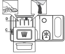
1. When measuring out the detergent refer to the mentioned earlier information to add the proper quantity. Inside the dispenser **D**, there are indications to help the detergent dosing.
