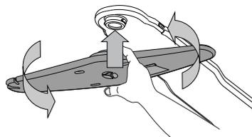
The top spray arm may be removed by pressing it up and then rotating it anti-clockwise. Mounting back the spray arm is by pulling it upwards and rotating it clockwise.
