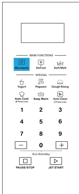
To cook **WITH** microwave power individually, press the Microwave button repeatedly to select a cooking power level, then press **+-** button to set a desired cooking time. The longest cooking time is 90 minutes.
