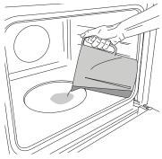
To start the Steam function, pour 200 ml of drinking water in the oven bottom. Select the function turning clockwise the selection knob on the relevant icon, and the thermostat knob in any position between 160 and 180°C (as suggested by the icon). The function will start and the display will show the current time of the day. No preheating is needed. To end the cooking, turn the selection knob on **0** position. During
