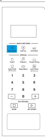
**Το cook with** microwave power individually, press the Microwave button repeatly to select a cooking power level, then press +/- button to set a desired cooking time. The longest cooking time is 90 minutes.
